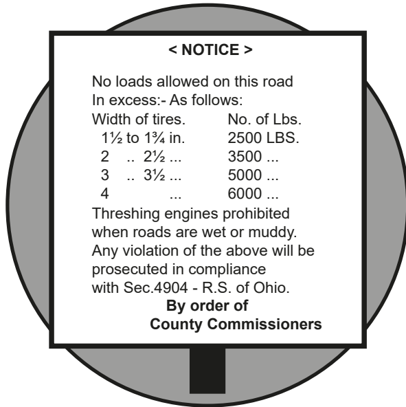
Figure 4.27: A road limit was one answer to the problem of heavy trucks breaking up the road surface
